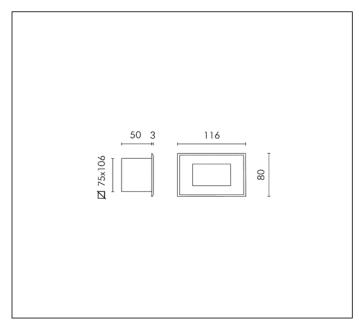
MODULES LED 3000K 230V CRI 80 Rated luminaire luminous flux: 28lm Rated input power: 1.3W Luminaire efficacy: 22lm/W 220÷240V 50/60Hz
