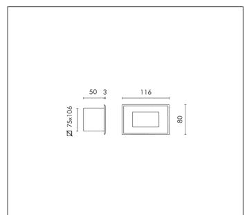
MODULES LED 6000K 230V CRI 75 Rated luminaire luminous flux: 40lm Rated input power: 1.3W Luminaire efficacy: 31lm/W
