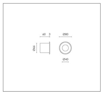
MODULES LED 3000K 230V CRI 80 Rated luminaire luminous flux: 28lm Rated input power: 1W Luminaire efficacy: 28lm/W
