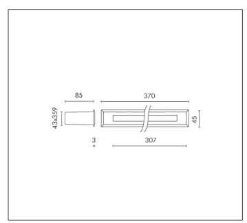
MODULES LED 3000K 230V CRI 80 Rated luminaire luminous flux: 56lm Rated input power: 2.4W Luminaire efficacy: 23lm/W 220÷240V 50/60Hz
