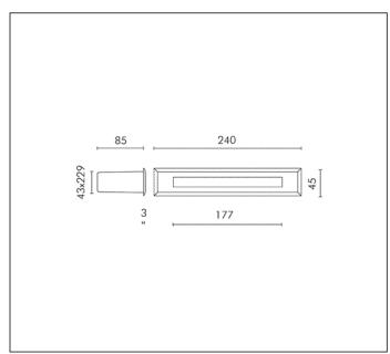
MODULES LED 3000K 230V CRI 80 Rated luminaire luminous flux: 28lm Rated input power: 1.3W Luminaire efficacy: 22lm/W
