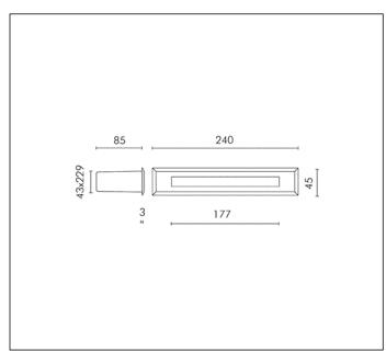
MODULES LED 6000K 230V CRI 75 Rated luminaire luminous flux: 40lm Rated input power: 1.3W Luminaire efficacy: 31lm/W
