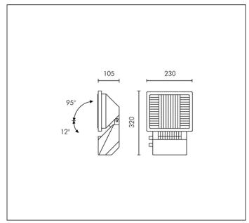
HIT-DE 150W CLEAR Rx7s 13250lm Rated luminaire luminous flux: 8215lm
