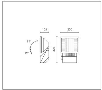
HIT-DE 70W CLEAR Rx7s 6500lm Rated luminaire luminous flux: 4680lm
