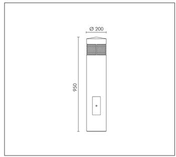
HIT-CE/S 70W CLEAR E27 6300lm Rated luminaire luminous flux: 1134lm
