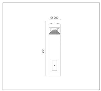
HIT-CE/S 70W CLEAR E27 6300lm Rated luminaire luminous flux: 2331lm
