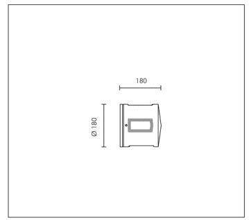
HIT-TC CRI 35W G8,5 3300lm Rated luminaire luminous flux: 429lm
