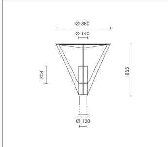
HIT-CRI 70W CLEAR G12 6600lm Rated luminaire luminous flux: 2442lm
