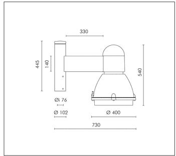
HIT-CE/S 70W CLEAR E27 6300lm Rated luminaire luminous flux: 4788lm
