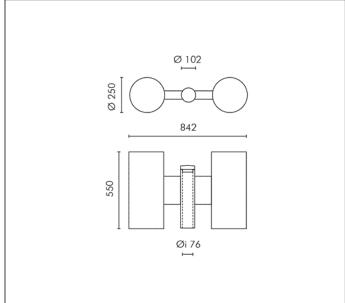
2x HIT-DE 70W CLEAR Rx7S 13000lm Rated luminaire luminous flux: 7150lm
