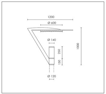
HIT-CRI 150W CLEAR G12 14000lm Rated luminaire luminous flux: 6440lm
