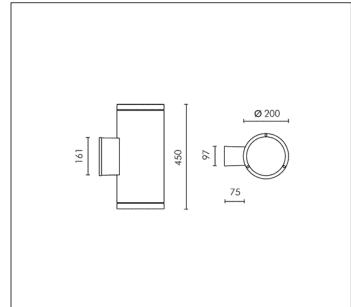
2x HIT-CRI 70W CLEAR G12 13200lm Rated luminaire luminous flux: 6336lm
