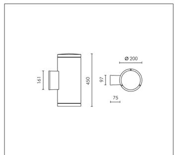
TC-TEL 26/32/42W Gx24q-4 3200lm Rated luminaire luminous flux: 1312lm
