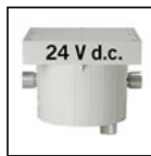
S.3665 JUNCTION BOX WITH POWER SUPPLY 70W 240V/24V c.c. IP65 power supply for: N°4 Micropool LED** o N°3 Minipool LED* or N°2 Pool LED maximum load capacity 500Kg Dimensions 300mm x300mm x230mm ** = require 2 x S.3670 additional cable gland * = require 1 x S.3670 additional cable gland
