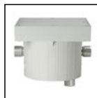
S.3660 JUNCTION BOX IP65* Junction box with cable glands for 3 cables IN (possibility of 3 more cables IN with S.3670 accessories) Maximum load capacity 500Kg Dimensions 300mm x300mm x230mm
