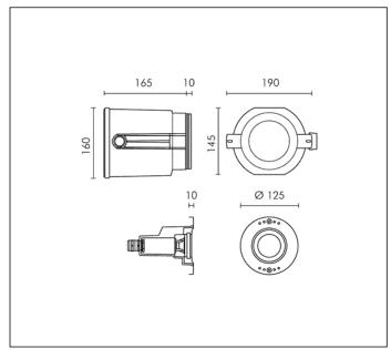
1 MODULES LED 6000K 24V 283lm CRI 70 Rated luminaire luminous flux: 140lm
