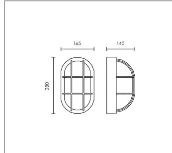
TC-DEL 18W G24q-2 1200lm Rated luminaire luminous flux: 516lm
