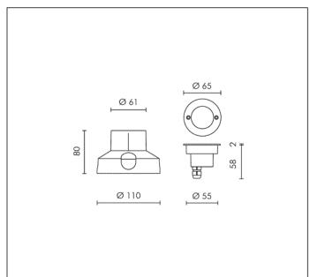
MODULES LED 4000K 24V c.c. CRI 90 Rated luminaire luminous flux: 30lm
