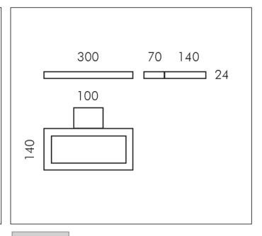
1 MODULES LED 4000K 230V 1944lm CRI 90 MacAdam step 3 Rated luminaire luminous flux: 1380lm Rated input power: 18W Luminaire efficacy: 77lm/W
