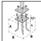
**S.2849****PLANTED ROOT for CYLINDRICAL POLE**C= 200mm, D=200mm E=Ø80mm, h=407mm, h1=90mm and bolts in galvanized steel with M16 threads. Suggested reinforced concrete footstall dimension \*\*:
