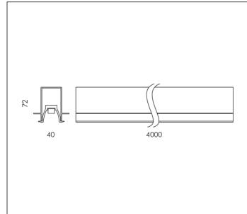
MODULES LED 3000K 24V 3200lm CRI 90 Rated luminaire luminous flux: 3200lm Rated input power: 46W Luminaire efficacy: 70lm/W
