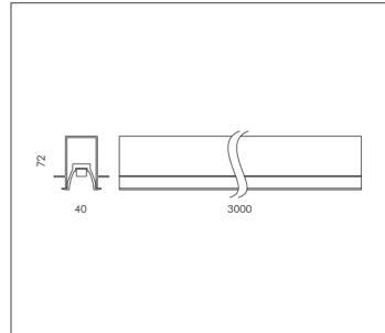
MODULES LED 3000K 24V 2400lm CRI 90 Rated luminaire luminous flux: 2400lm Rated input power: 34.5W
