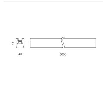
MODULES LED 3000K 24V 4800lm CRI 90 Rated luminaire luminous flux: 4800lm Rated input power: 69W Luminaire efficacy: 70lm/W
