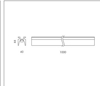
MODULES LED 4000K 24V 800lm CRI 90 Rated luminaire luminous flux: 800lm Rated input power: 11.5W
