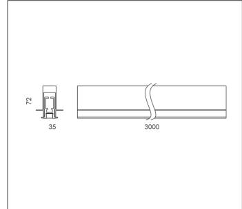
MODULES LED 4000K 24V 2400lm CRI 90 Rated luminaire luminous flux: 2400lm Rated input power: 34.5W
