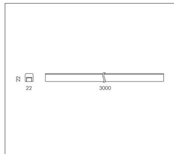
MODULES LED 3000K 24V 2400lm CRI 90 Rated luminaire luminous flux: 2400lm Rated input power: 34.5W
