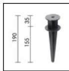
S.1014 GROUND STAKE In POLYPROPYLENE. Colour: black (code .09) The 35 mm upper part must stay above ground level, according to the norm.
