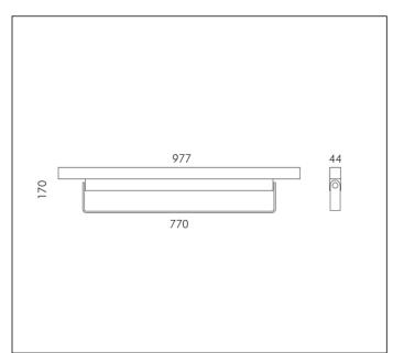
MODULES LED 4000K 230V 8140lm CRI 90 Rated luminaire luminous flux: 5652lm
