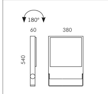
MODULES LED 3000K 230V 19905lm CRI 80 Rated luminaire luminous flux: 13812lm Rated input power: 147W
