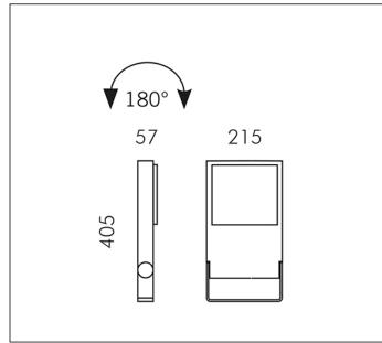
MODULES LED 3000K 230V 4524lm CRI 80 Rated luminaire luminous flux: 2844lm Rated input power: 35W
