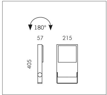
MODULES LED 4000K 230V 4649lm CRI 80 Rated luminaire luminous flux: 2923lm
