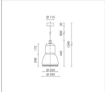
HIT-CRI 150W CLEAR G12 14000lm Rated luminaire luminous flux: 9660lm
