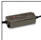
S.3402 REMOTE POWER SUPPLY DIMMABLE 40W IP67 Dimmable 1-10V for monochromatic LED 40W 240V/24V DC IP67 The Total power of all connected luminaires may not be higher than the power of the driver. Dimensions 150x53x35mm
