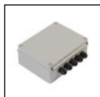
S.3422 BOX WITH DIMMABLE REMOTE POWER SUPPLY 50W 1-10V IP55 50W 240V/24V d.c. 1-10V 5 Exit The Total power of all connected luminaires may not be higher than the power of the driver. Dimensions 260x260x100mm IP55
