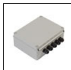
S.3420 REMOTE BOX NOT DIMMABLE 100W IP55 POWER SUPPLY 240V/24V d.c. 5 Exit Dimensions 260x260x100mm The Total power of all connected luminaires may not be higher than the power of the driver. IP55
