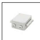
S.3401 BOX IP 55 WITH ELECTRONIC POWER SUPPLY 10W 24V D.C. (Electronic power supply included) Dimensions: &nbsp;230 x 210 x 80 mm. Cable IN: &nbsp;&nbsp;&nbsp;&nbsp;&nbsp;&nbsp;2 with cable glands PG11 Cable OUT: 6 with cable glands PG11 IP55 CLASS II The Total power of all connected luminaires may not be higher than the power of the driver.
