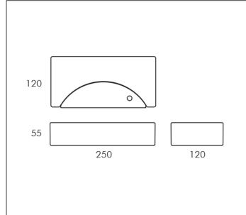
MODULES LED 3000K 300lm CRI 80 Rated luminaire luminous flux: 120lm
