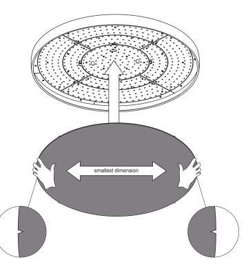
Be careful not to damage the LEDs when inserting the diffusor.
