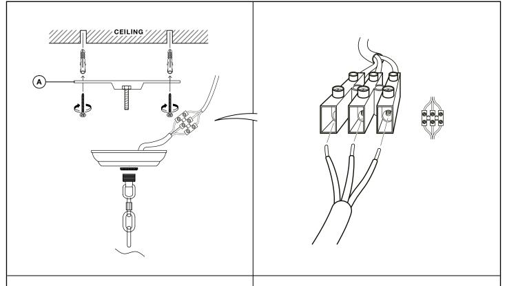
Turn off the electricity supply at the main circuit panel before installing. Do not connect the electricity supply until your luminaire is fully assembled and installed.
