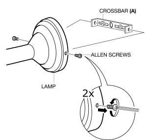
Turn off the electricity supply at the main circuit panel befor installing. Do not connect the electricity sypply until your luminaire is fully assembled and installed.
