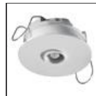
Extension movement detector white, recessed. To be used when the area to be covered is bigger than 6,00x5,00m by height 2,50m. To be connected to one of the outputs of the INTERACTIVE-DALI controller. No extra mains connection required. M074130
