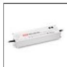
Electronic power supply. IP67. Input voltage range: 90- 264VAC / 47-63Hz. Output voltage: 48VDC. Protection against overcurrent, overvoltage, short- circuit and overtemperature, with automatic restart. - 320W. For feeding up to a total 300W. 252x90x44mm. M076100
