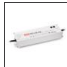
Electronic power supply. IP67. Input voltage range: 90-264VAC / 47-63Hz. Output voltage: 48VDC. Protection against overcurrent, overvoltage, short-circuit and overtemperature, with automatic restart. 100W. For feeding up to a total 90W. 220x68x38mm. M075000
