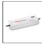
Electronic power supply. IP67. Input voltage range: 90-264VAC / 47-63Hz. Output voltage: 48VDC. Protection against overcurrent, overvoltage, short-circuit and overtemperature, with automatic restart. - 240W. For feeding up to a total 225W. 244x68x39mm. M075100
